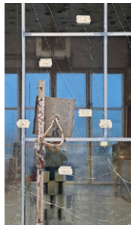
Fire Test temperature detection sensors for fire test on fixed frame
